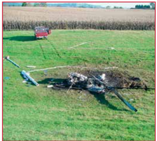
Vehicle tyre tracks can cause damage to witness marks, if an accident site is uncontrolled.
