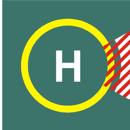
Figure 5-7. Helideck prohibited landing sector marking
