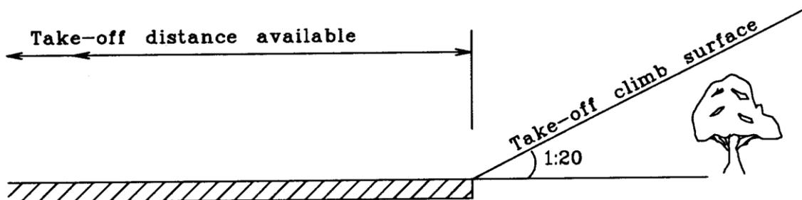
Figure 1. Obstacle free design take-off surface
