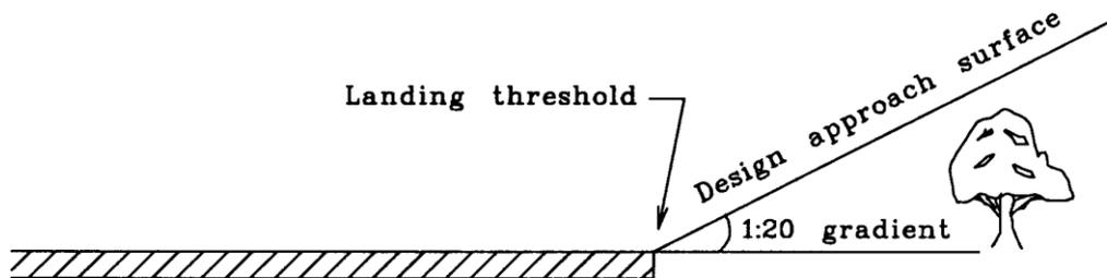
Figure 4. Aerodrome design approach surface - no obstruction
