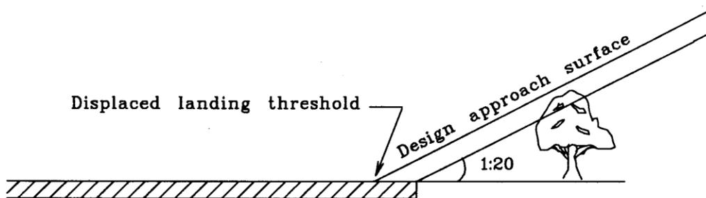
Figure 5. Aerodrome design approach surface - obstruction
