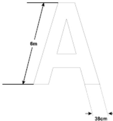
**Figure 1.** Agricultural operations aerodrome ground signal
