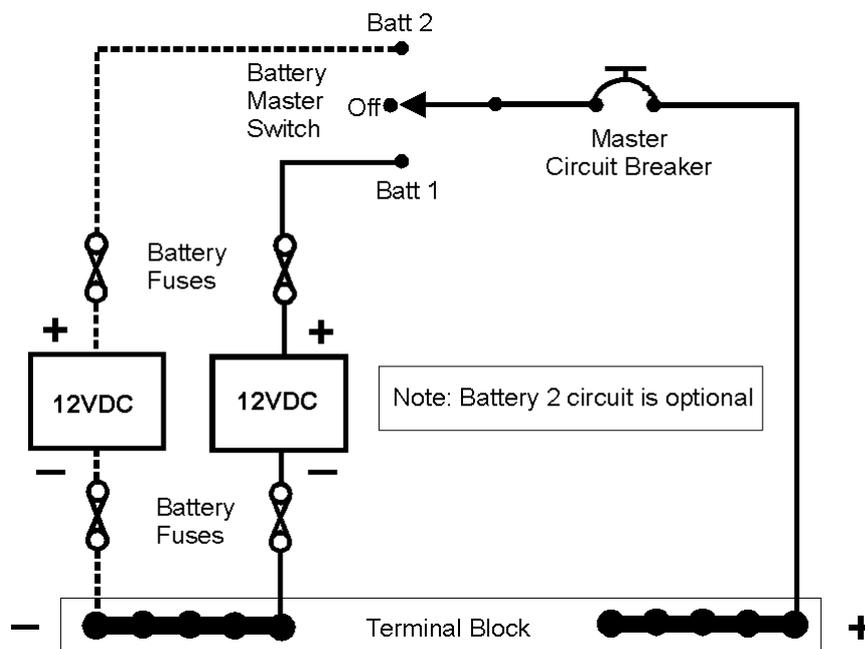
4.6. Placard the master switch, master circuit breaker, battery fuses and terminal block.
